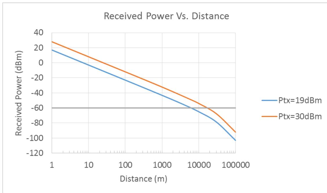
*3X range increase (6km vs. 18km) by increasing transmit power 11dB*
